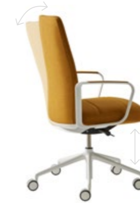
Synchronized mechanism. Swivel base on casters. Seat height adjustment with gas lift. Synchronized tilt movement of the seat and back. Four locking positions. Tension adjustment to user weight.
